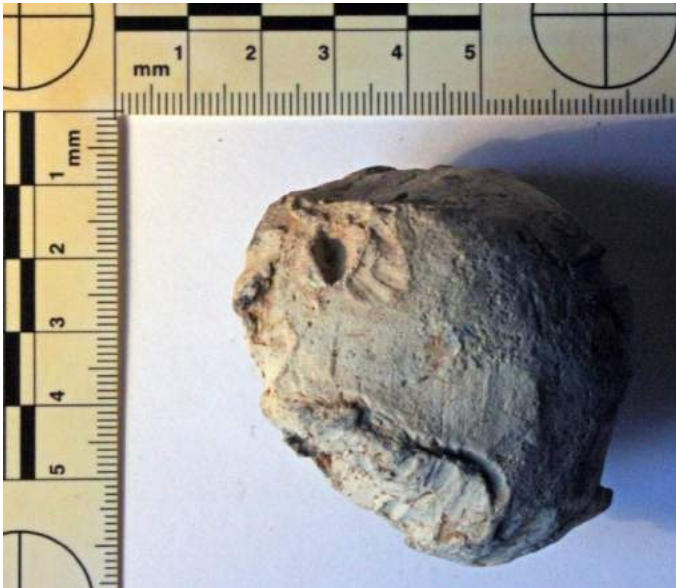
Figure 44: Image showing the degree of deformation of the ball, with a wide gouge and associated spalling of lead clearly overlapping the firing band.
