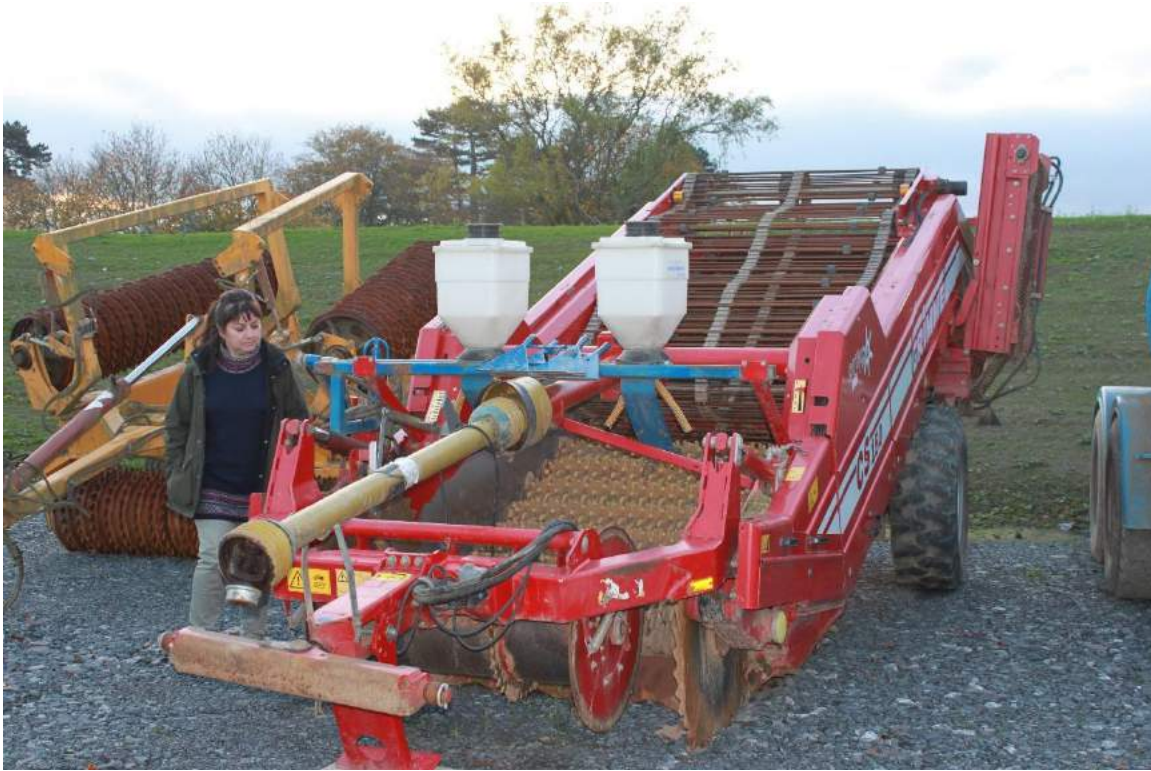
Figure 23: Destoning machinery used prior to planting potatoes.
