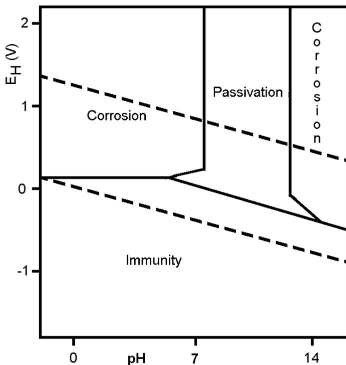
**Figure 9: Comparison of the iron and copper diagrams demonstrate why copper alloy condition is often better on a wide range of burial sites. However, metal stability, especially the formation of passivation layers are severely affected by the presence of chloride**
