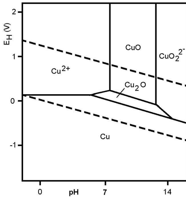
**Figure 8: Simplified Pourbaix diagram (Potential –pH) for copper-water at 25°C. (to left) Cu,  $Cu_2O$  and  $CuO$  are in solid phase, while  $Cu^{2+}$  and  $CuO^{2-}$  are in solution**
