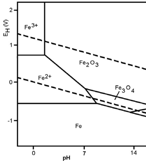
Figure 6: Simplified Pourbaix diagram (Potential –pH) for iron-water at 25°C. Fe,  $\text{Fe}_2\text{O}_3$  and  $\text{Fe}_3\text{O}_4$  are solids, while  $\text{Fe}^{2+}$  and  $\text{Fe}^{3+}$  are in solution<sup>22</sup>
