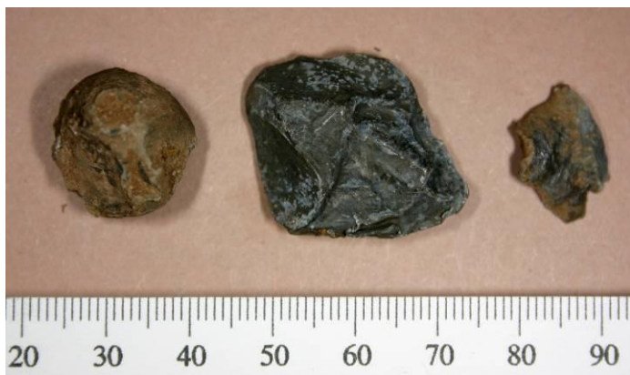
Figure 11: Case shot: though typically polygonal it can have part of the original round ball surface surviving (left) or be heavily distorted (centre). Fragments from impacting (right) might be found (Experimentally fired bullets)
