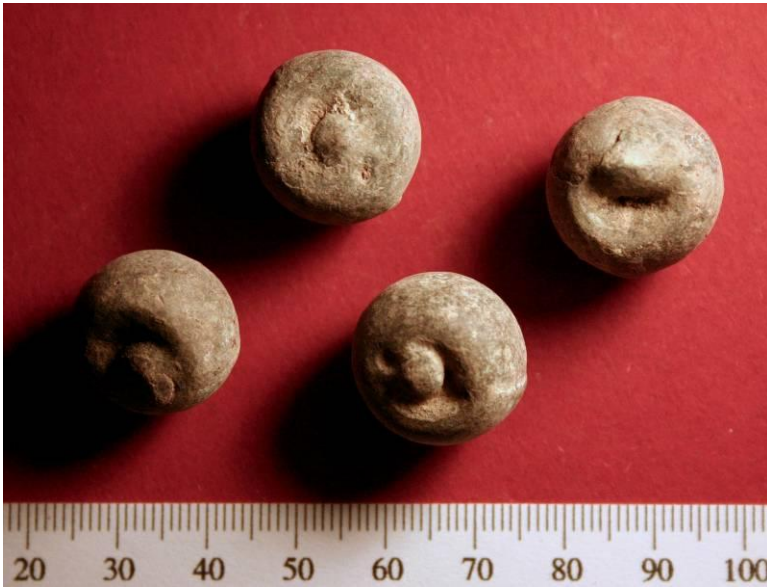
Figure 19: Poorly cast bullets where the mould was incompletely filled resulting in an incomplete sphere and lacking a sprue (Ballymore)
