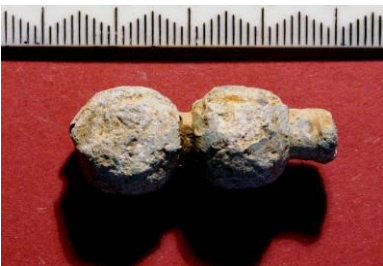
Figure 6: Dumbbell bullet with sprue intact, demonstrating manufacture in a double mould (Easton Maudit)
