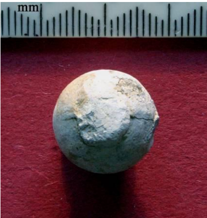
Figure 14: This sprue, sitting as always astride the mould line, here clearly visible as a slight offset, was left proud when cut or nipped. The remnant sprue has subsequently been swaged over, possibly by bumping during transport (Edgehill 564)
