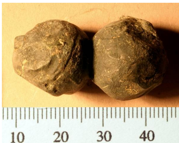
Figure 12: Two case shot bullets welded together during firing and showing a high degree of melting of the bullet surfaces, due to the high temperatures in the barrel of the artillery piece (experimentally fired bullets)
