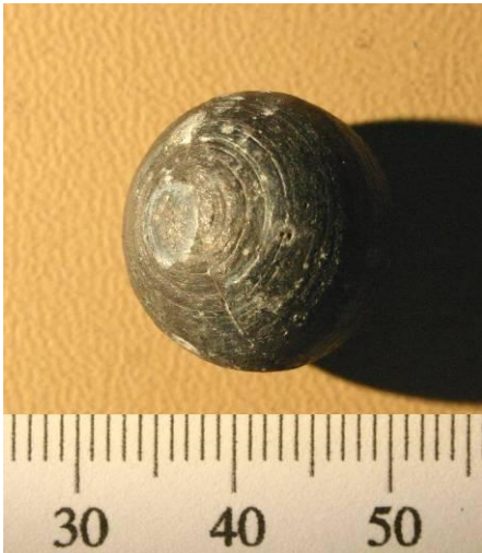
Figure 21: Latitudinal lines centering on an axis through the sprue, possibly reflecting the original cutting of the mould with a router (Swan bullet 38)
