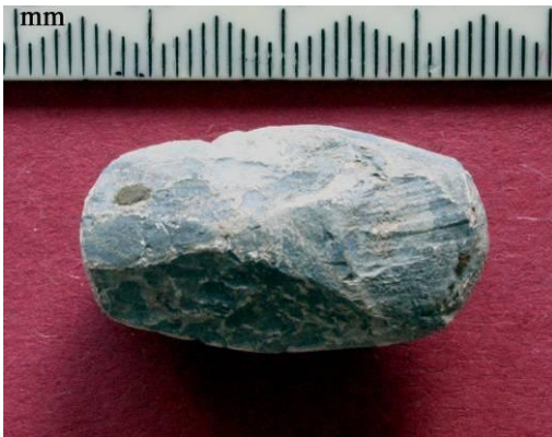
Figure 4: Irregular slug showing a number of separate facets (Edgehill 512)
