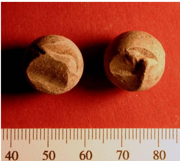
Figure 16: Careless cutting of the sprue has left partial deep cuts and has also removed a substantial part of the sphere of the ball, thus significantly affecting bullet weight. The striations from the tool used can be seen on the lower face of the left bullet (Ballymore)
