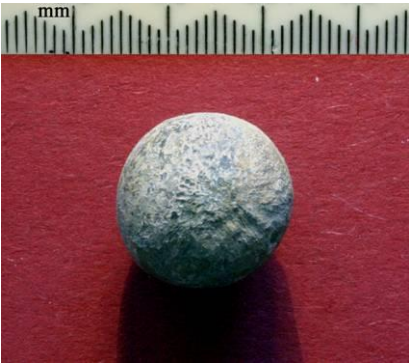
Figure 25: Pitting and faintly radial striation on the lower hemisphere of the bullet (Edgehill 680)
