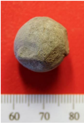
Figure 22: Paring represented by a series of flat surface along the mould line, where the flash has been removed by cutting (Vasa 17154.48)
