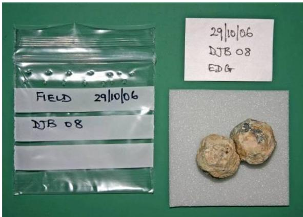
**Figure 2: Perforated find bag partially labelled plus Tyvek label and foam support**
