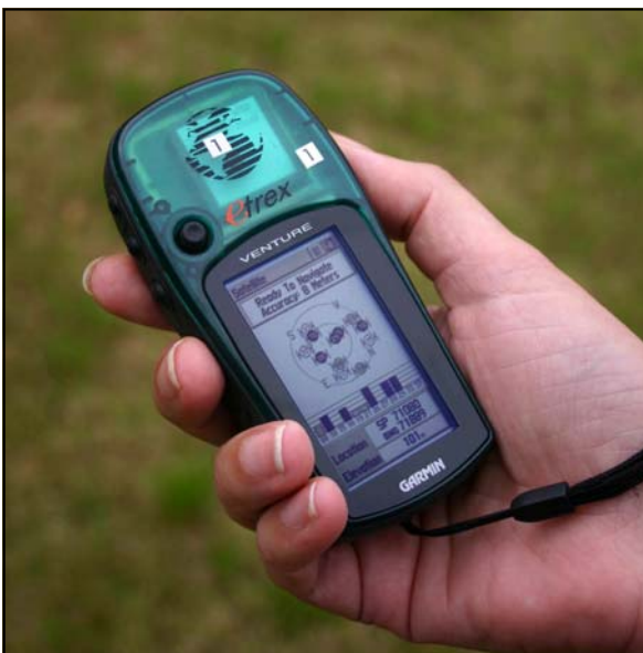
Figure 8: 'Garmin Etrex Venture' GPS units, now costing well under £150 each, with their essential protective cases, are attached to each of the metal detectors. They are used to record the 'waypoint' location of every find and to record the track followed by the detectorist. The data is then downloaded using 'GPS Utility' software and imported into 'MapInfo' GIS for mapping and analysis.
